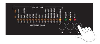
When the valve is heated, the yellow light will go out and the green will come on. The valve is now ready, tap the valve gently with a pencil to test microphony. Note: If there is any noise present in the valve some LEDs will illuminate prior to tapping.
