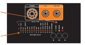
For example, power valves are graded with their emission and control grid performance as primary factors, whereas pre-amp valves are graded with different parameters to reflect their role in signal amplification and phase splitting applications. If the valve is faulty or worn, then this will be indicated at the end of the test.
