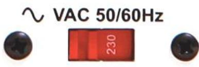
The voltage selector switch and mains fuse are factory set for the region in which your amplifier is intended to be sold. Do not tamper with this switch without express permission from Orange Music Electronic Company Ltd.
