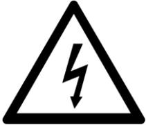
The lightning flash with arrowhead symbol, within an equilateral triangle, is intended to alert the user to the presence of un-insulated 'dangerous voltage' within the product's enclosure that may be of sufficient magnitude to constitute a risk of electric shock to persons. Terminals labelled as "Speaker Outputs" must be connected to a speaker cabinet of the designated load rating using an un-shielded two conductor cable for speaker use at all times during operation
